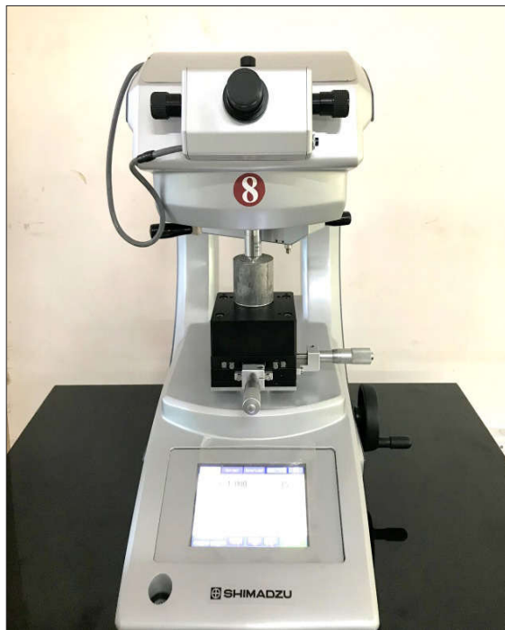
Fig. 2. Specimen loaded on (Shimadzu) hardness tester
