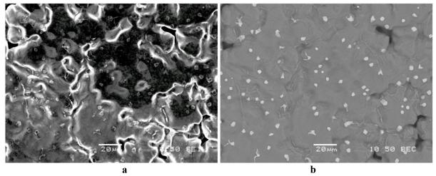
**Fig. 4.** SEM image from the general view of the inner surface of an entrapped UHP argon bubble in AZ91D alloy a) SE image from surface film, b) BE image from the same area showing Al-Mn intermetallic particles.
