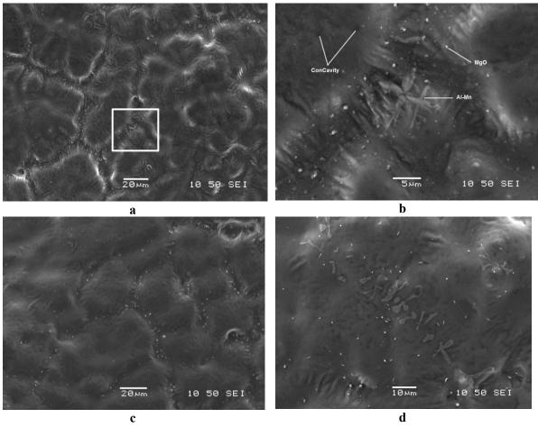
Fig. 7. SEM images of the inner surface film formed on an entrapped bubble of air/3.5%SF<sub>6</sub> mix in AZ91D and AM60B alloys: a,b) Secondary electron images showing typical areas in AZ91D alloy, c,d) SE images of the surface film morphology in AM60B alloy.
