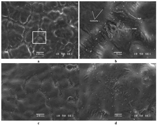
**Fig. 8.** SEM image from the general view of the inner surface of an entrapped UHP argon bubble in AM60B alloy: a) SE image from general view of the surface film, b) magnified view from clean part area, c) magnified view of a thick rough oxide patch area, and d) EDS spectra from clean and oxide patch areas..
