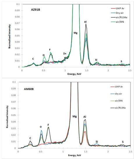
Fig. 2. Representative EDS spectra of the early surface films of bubbles formed in molten AZ91D alloy and AM60B alloy using different bubble gas atmospheres. These spectra have been normalized to the Mg  $K_{\alpha}$  peak and the relevant peaks identified for AZ91D and AM60B.
