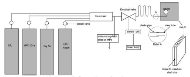
Fig. 1. Schematic diagram of the experimental arrangement
