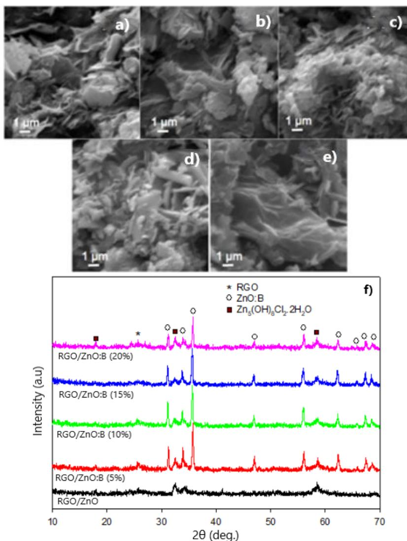
**Fig. 3.** SEM images of RGO/ZnO:B composites with different boron concentrations: a) 0 wt.% b) 5 wt.% c) 10 wt.% d) 15 wt.% e) 20 wt.% and f) XRD pattern of RGO/ZnO:B composites with different boron concentrations.
