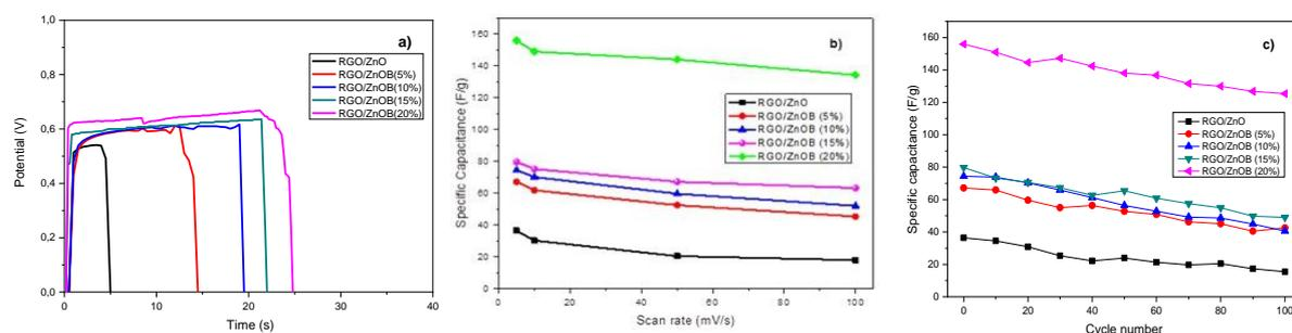
**Fig. 5.** a) The charge/discharge curves of Graphite/PTFE/ RGO/ZnO:B electrodes b) The changes in capacitance value under different scanning rates, and c) The changes in capacitance values according to the number of cycles.
