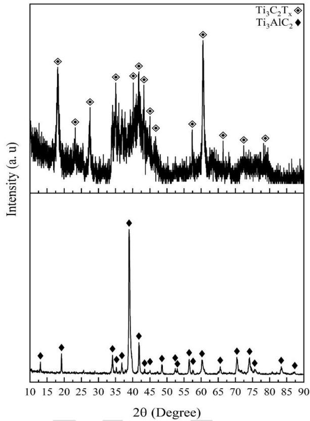
Fig.1. X-ray diffraction patterns of  $Ti_3AlC_2$  MAX phase a) before and b) after etching process in HF solution for 24 h.
