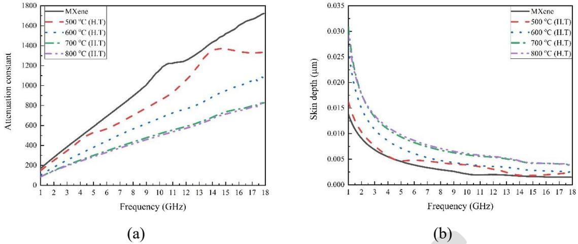
Fig. 7. The changes in a) attenuation constant and b) skin depth in relation to frequency (within 1-18 GHz) for  $Ti_3C_2T_x$  MXene phase before and after annealing process at different annealing temperatures.
