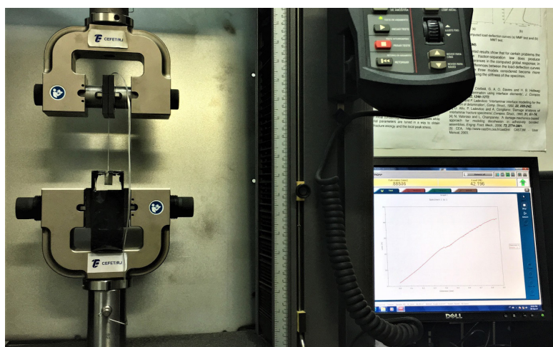
Fig. 3. Instron machine and RTC clamp
